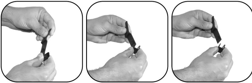
2. Loosen or remove front rail screw, and slide ABR into desired position beneath rail. Re-tighten front rail screw.
