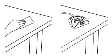
5. To change the location of the charging dock, firmly grip the base of the charging dock and pull up. Apply the dock base to the new area and press down firmly, making sure that the surface you are reattaching to is clean.
