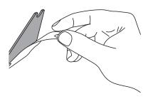
Making sure the anti-slip pad is aligned with the bottom of the charging dock, press the exposed side down onto the bottom of the charging dock.
