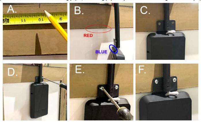
8. Attach Charging Cord: Untie charging cord and keep the twist tie (Part D). A.& B. Plug cord into battery pack C. Place cord clip (Hardware Packet) on to female end of the cord. Select the best side and location to mount the charging cord on, based on convenience to a power outlet. D. Screw the cord clip to the frame, making sure it is concealed when not in use. F. Tie excess cord together with twist tie to keep it out of the way.
