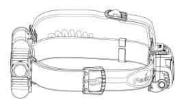
Attach the top headband to the headlamp holder and the battery case as shown.
